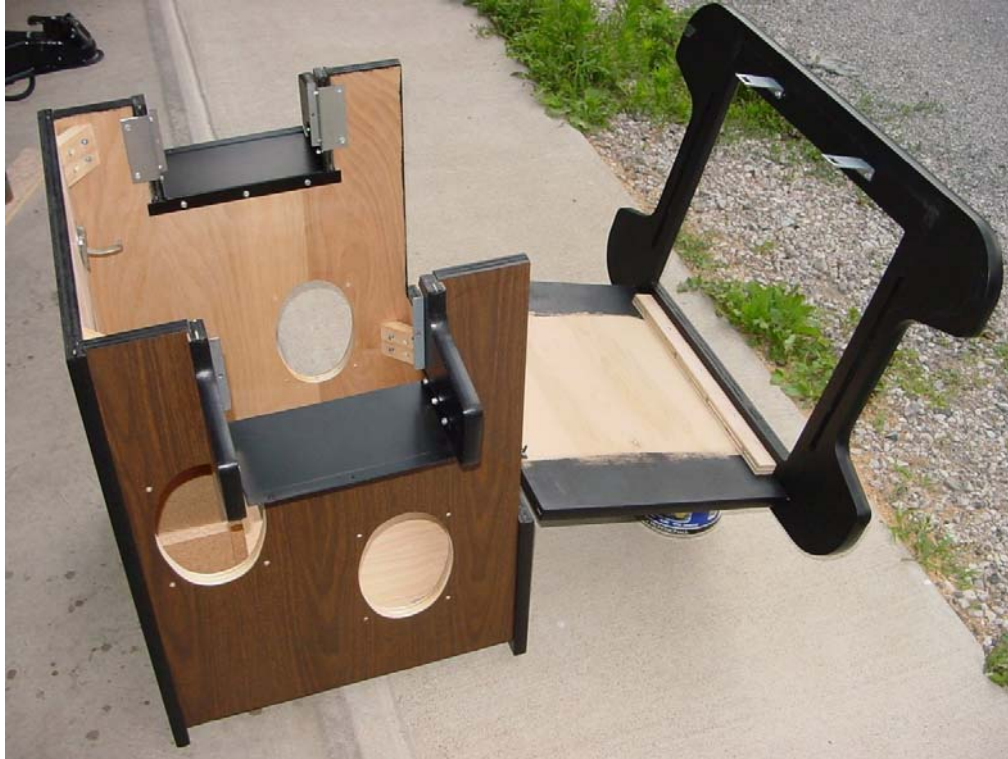
Here is what the cabinet looks like with the control panels, top, latches and coin door installed.
