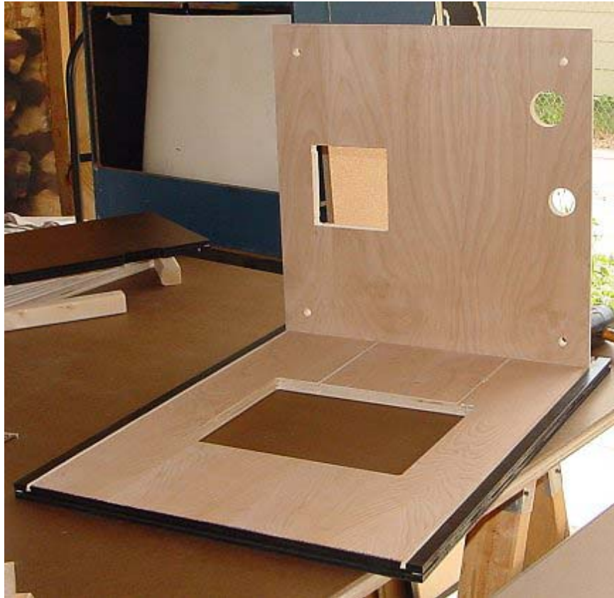
Assembling the cabinet front with the cabinet bottom.
