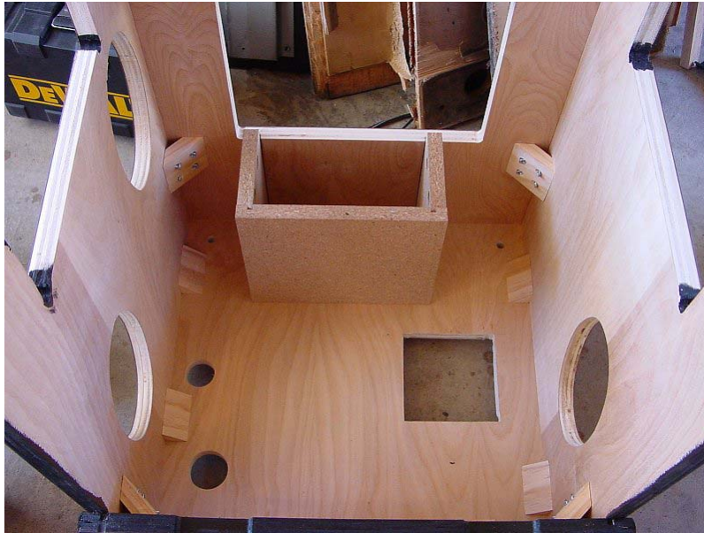
Coin box is installed. Notice the lower corner gussets are glued in place.
